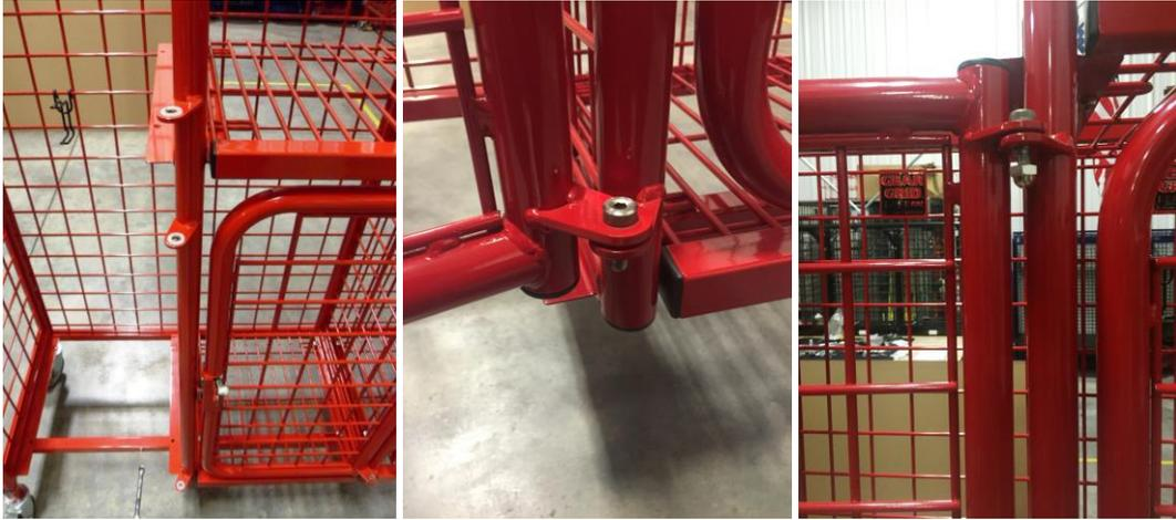
Step 6. Attach striker bolt. Per side, grab (2) striker bolts and thread into side tube, then tighten striker bolts (see photo).
