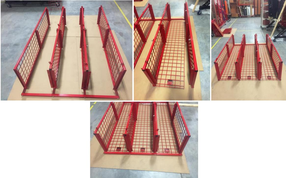
Step 4. Attaching shelves. Grab (1) shelf, (4) 1"x5/16-8 carriage bolts, and (4) 5/16-18 nuts. Insert carriage bolt into shelf and through bracket, now thread on nut. Do these steps for all shelves. (There are (3) shelves per opening) Do not tighten hardware until all doors are installed. Leaving hardware loose will allow you some adjustability in the side panels for centering doors. Once your doors are centered you may now tighten hardware.
