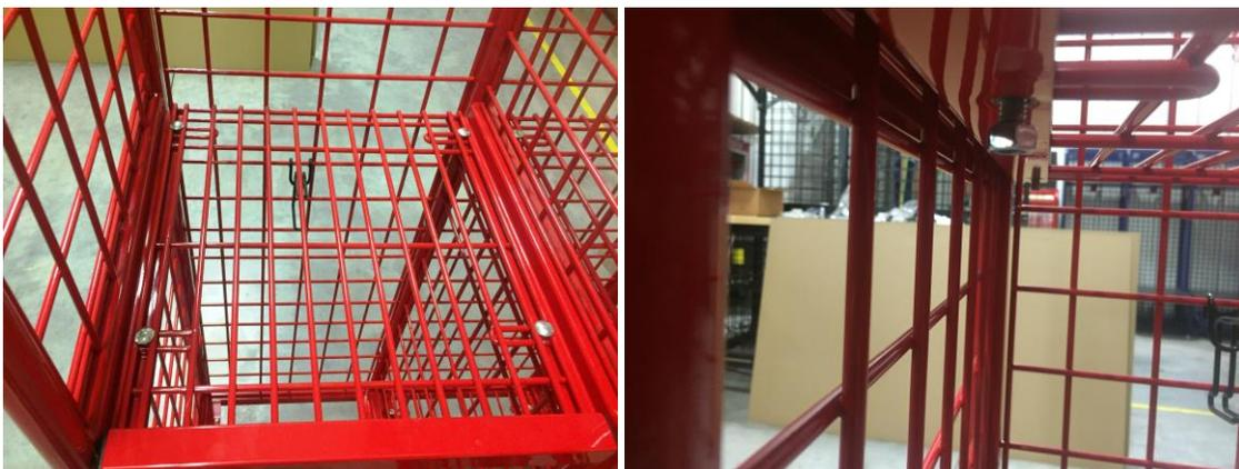
Step 5. Attaching locker doors to side tubes. First grab (4) .380 x .750 x .062 nylon washers and place them on the tabs of the side tubes. (See photo) Next grab (1) locker door and (2) 1/2" shoulder bolts and insert bolts through door tabs and attach door to side tube. (See photo) Next, grab (4) acorn nuts and thread onto shoulder bolts. (See photo) now tighten hardware. Do these steps for all doors.
